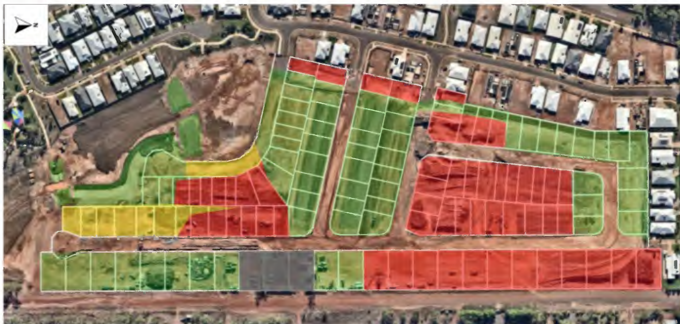
Figure 10: Fill Areas at Finished Surface Level and Earthworks progress (Based on Level 1 Testing)
