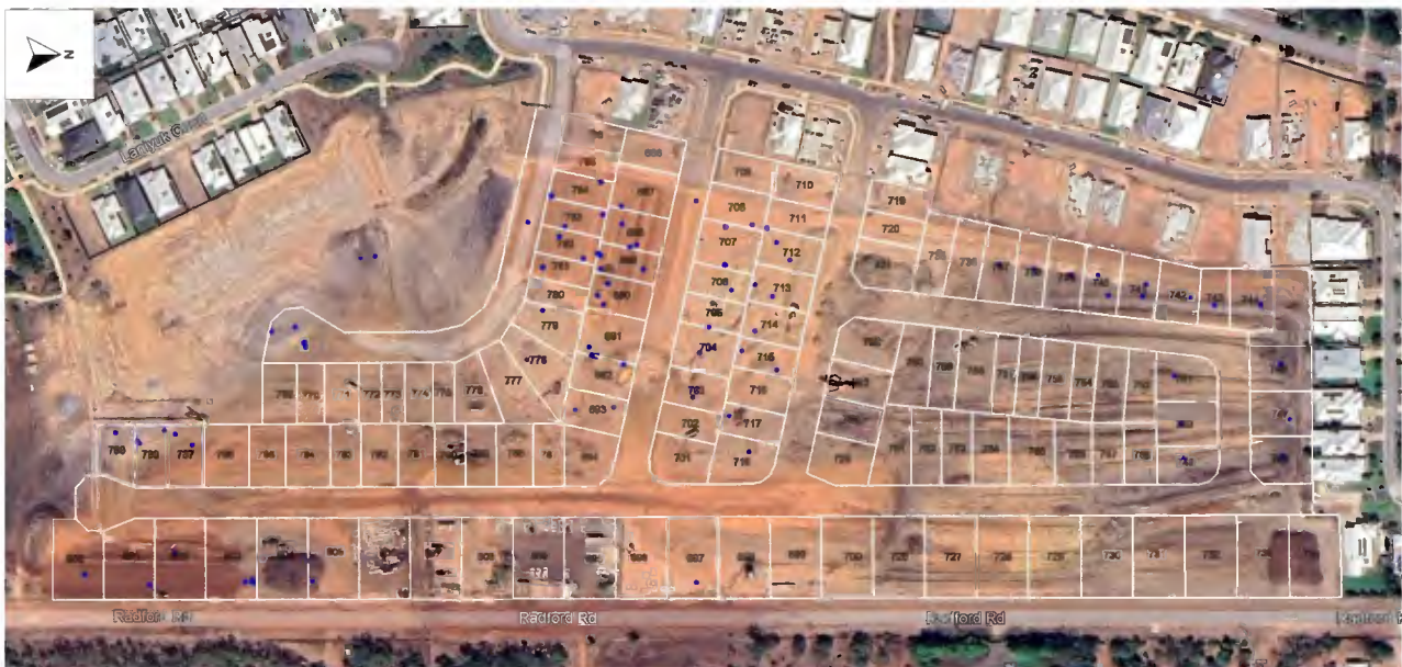
Figure 9: Approximate Compaction Testing Locations
